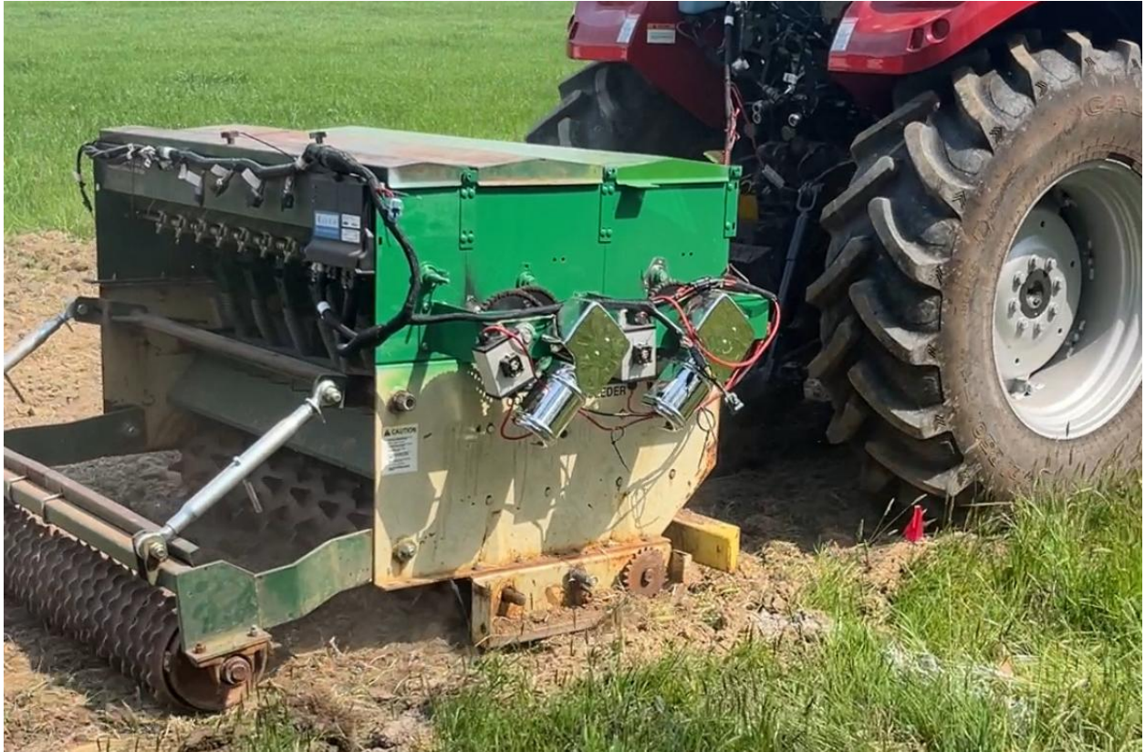
Figure 3. Seeder with RCM and electric drive components during initial field testing.
